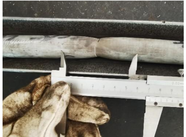
Dimension inspection after tensile test
